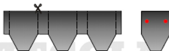
Picture Nr. 7- Cutting of the ridges
